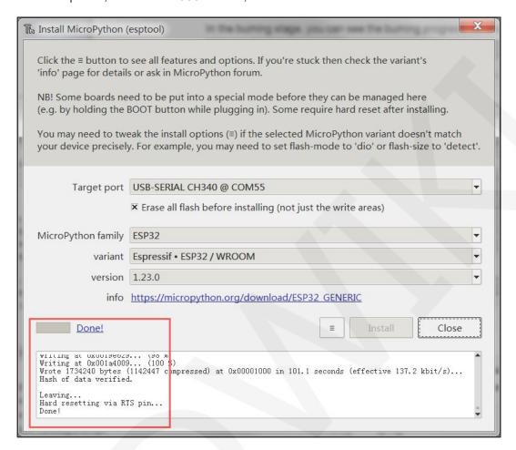
Figure 4.18 The ESP32 MicroPython firmware has been burned online
