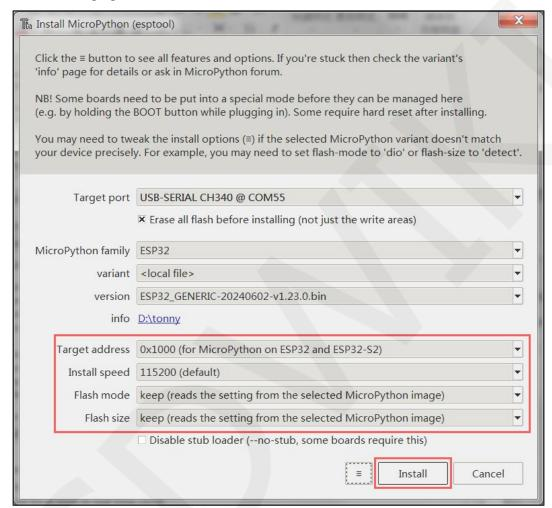
Figure 4.13 Configure the ESP32 module
