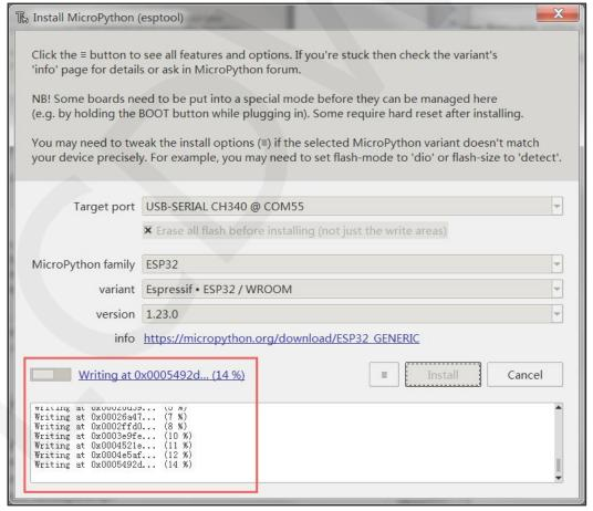
Figure 4.17 ESP32 MicroPython firmware is burned online
