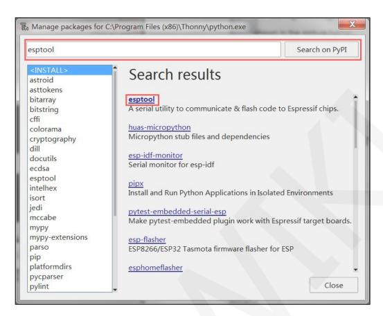
Figure 4.8 Install the esptool software package
