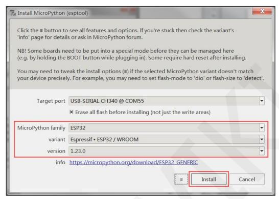
Figure 4.16 ESP32 MicroPython firmware online burning configuration
