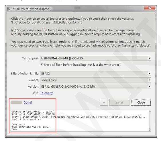
Figure 4.15 ESP32 MicroPython firmware has been burned
