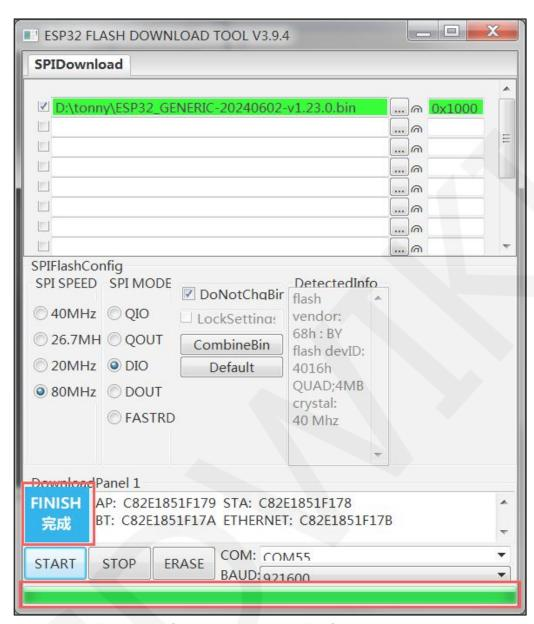
Figure 4.22 flash download tool The firmware is burned
